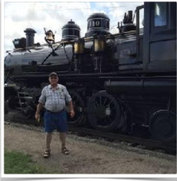
Number 110 was the flagship stem locomotive of the LRR—Little River Railroad. It was special ordered by Colonel W. B. Townsend, so as to combine the power of a logging (Shay) locomotive with the speed of a traditional passenger train locomotive. It was further distinguished by the fact that it was the smallest Pacific type engine ever built in the United States to run on standard gauge track.
